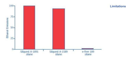
Silquest A-1589 silane (Disulfide silane), Silquest A-1891 silane (Mercapto triethoxy silane), and e-free 189 silane
